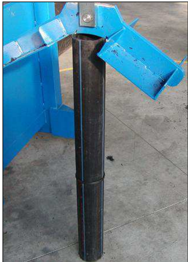
Figure 6 .Supporting the pipe's clamps
